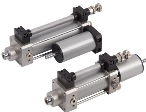
CIC hydraulic speed regulator, is an oil system with closed circuit which has to be connected to a pneumatic cylinder in order to obtain an adjustable slowing down of the stroke.
