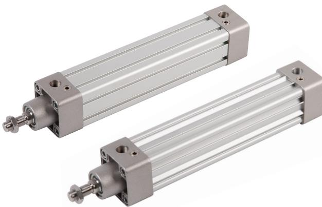
CY and CZ series cylinders are produced complying the ISO 15552 norm: they have bores between 32 and 125 mm. Particularly indicated where precision is important, they are available in different versions: double effect, cushioned and magnetic.
