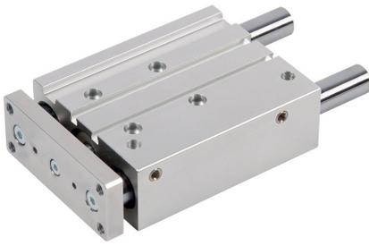
Guide compact cylinders are CIC's top of the range. This linear actuator offers a very high robustness combined with very small dimensions. It has a central pneumatic cylinder and the guiding system is based on rods with very big diameter which move on self lubricant brass bearings or balls sleeves. It is possible to mount the cylinder in different positions and to change the orientation of the feeding devices, according to all customer needs. Moreover, it is possible to mount magnetic sensors.
